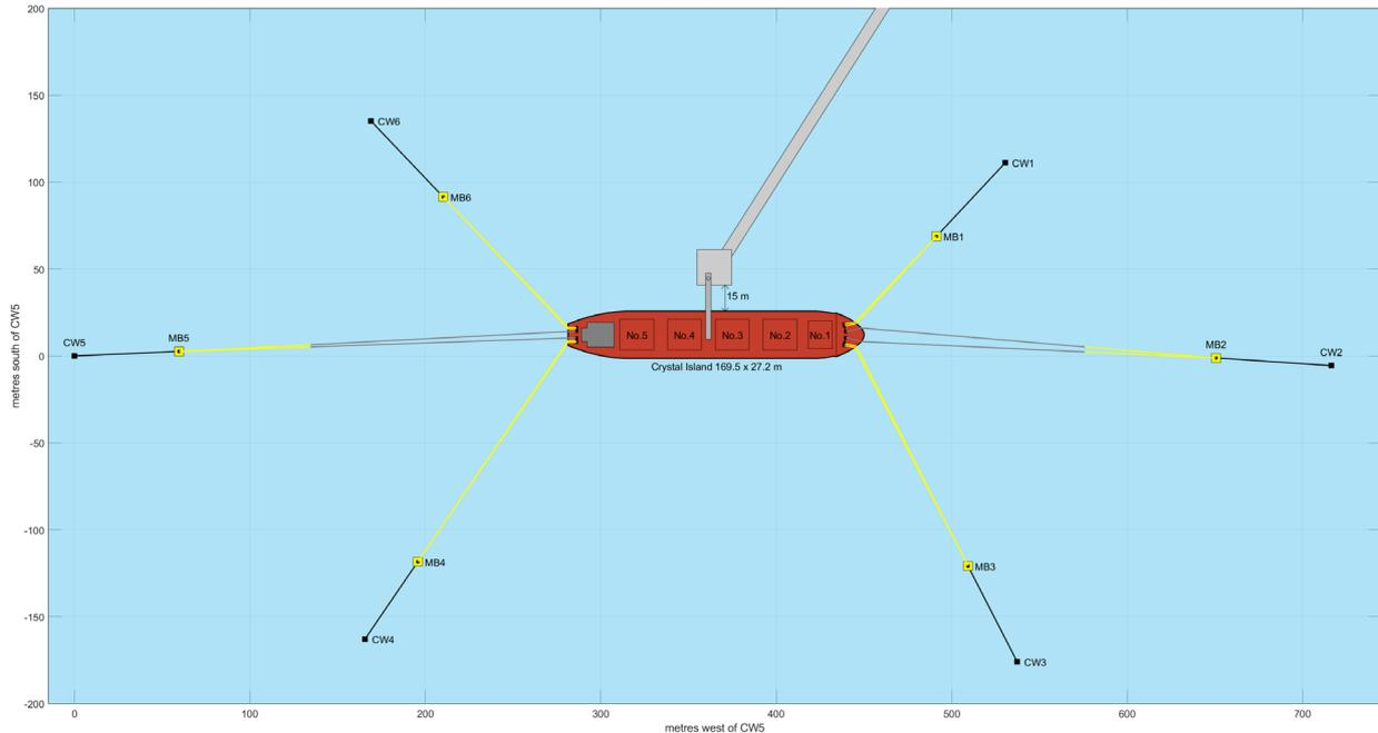
Figure 8 Mooring arrangement for Crystal Island test case, total 12 mooring lines. Yellow lines are polypropylene; grey lines are steel wire; black lines are anchor chain.
