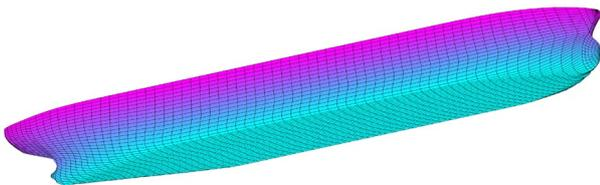
Figure 6 4256-panel surface mesh for Crystal Island, as used for WAMIT calculations
