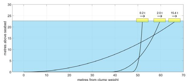
Figure 7 Mooring buoy position, as a function of horizontal load, for MB2. 15.4 tonnes corresponds to the chain lift-off tension in this case.
