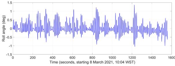
Figure 5 Roll motions for Panamax ship Alam Kekal, while loading No. 5 Hold as shown in Figure 4, with measured swell  $H_S = 1.5$  m,  $T_P = 15.8$  s and  $D_P = 270^\circ$ . Roll motions measured from the bridge with iPhone 12 and SensorLog software.
