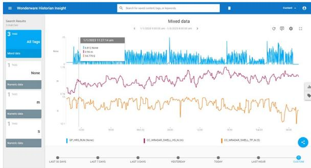
Figure 10 Real-time data monitoring for visit of MV Enishi (1-3 January 2023). (Top) Measured load on MB3; (Middle) Measured swell  $H_s$ ; (Bottom) Measured swell  $T_p$ .
