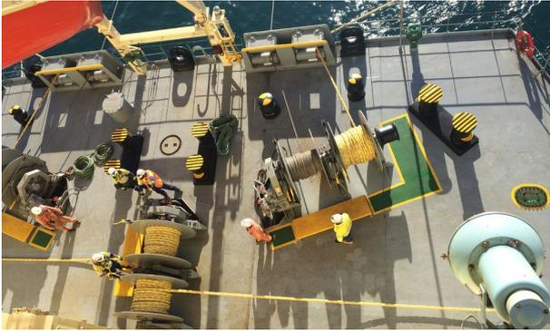
Figure 9 Port-supplied steel wire stern lines and Danstrong aft breast lines, as used for Crystal Island test case. Shown here on Alam Kekal, March 2021.
