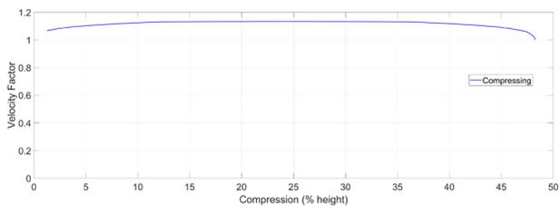
Figure 9 Calculated Velocity Factor for SCK400 fender during compression phase of cyclic load testing
