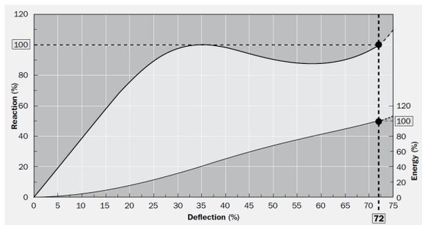
Figure 15 Load-compression curve for Trelleborg Super Cone fenders, as used at Geraldton Berth 5
