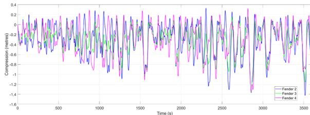
Figure 4 Fender compressions for Sea Diamond test case, including negative compressions (distance off each fender)
