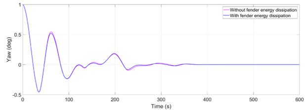
Figure 17 Yaw free decay test, without and with fender energy dissipation
