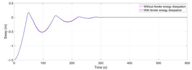
Figure 16 Sway free decay test, without and with fender energy dissipation
