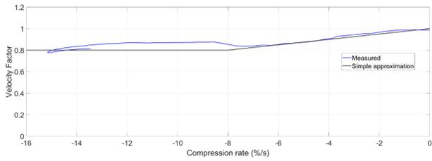
Figure 13 Calculated Velocity Factor for SCK400 fender while decompressing, plotted against compression rate. A simple approximation to the measured curve is also shown.
