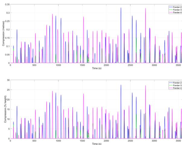
Figure 3 Fender compressions for Sea Diamond test case. Fenders are numbered as shown in Figure 2. (Top) Compression in metres; (Bottom) Compression as percentage of fender height (1.200m).
