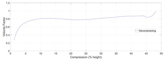
Figure 11 Calculated Velocity Factor for SCK400 fender, during decompression phase of cyclic load testing
