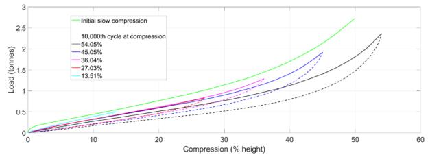
Figure 7 Compression-decompression curves for 55.5 mm cell fender. Solid line = compression. Dashed line = decompression. Data from ([7], Fig. 2 and Fig. 7).
