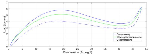
Figure 10 Compression-decompression curve for Trelleborg SCK400 cell fender during cyclic load testing, together with equivalent slow-speed compressing curve
