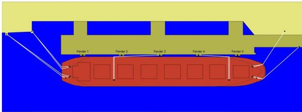
Figure 2 Mooring arrangement, for Sea Diamond at Geraldton Berth 5, 1<sup>st</sup> – 2<sup>nd</sup> Oct 2015. Fenders 2, 3 and 4 are in contact with the hull.
