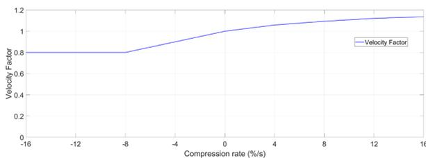
Figure 14 Velocity Factor for SCK400 fender, as a function of compression rate
