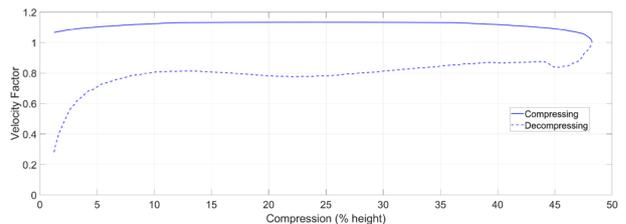
Figure 12 Velocity Factor for SCK400 fender, over complete compression-decompression cycle
