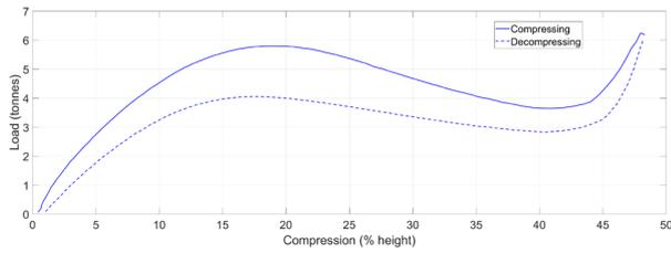
Figure 6 Compression-decompression curve after 1778 cycles, for Trelleborg SCK400 cell fender. Data from [Trelleborg14, Fig. 5].
