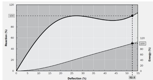
Figure 8 Load-compression curve for Trelleborg cell fenders, from ([8], p.21).
