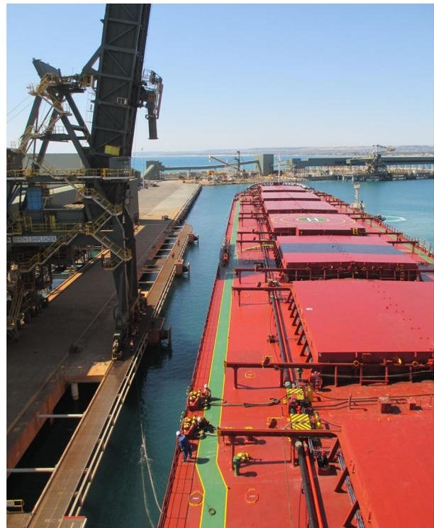
Figure 1 Sea Diamond arriving at Geraldton Berth 5, 1<sup>st</sup> Oct 2015. Trelleborg Super Cone fenders and low-friction facing are visible.
