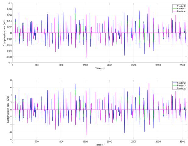
Figure 5 Fender compression rates for Sea Diamond test case. (Top) Compression rate in metres per second; (Bottom) Compression rate as percentage of fender height, per second.
