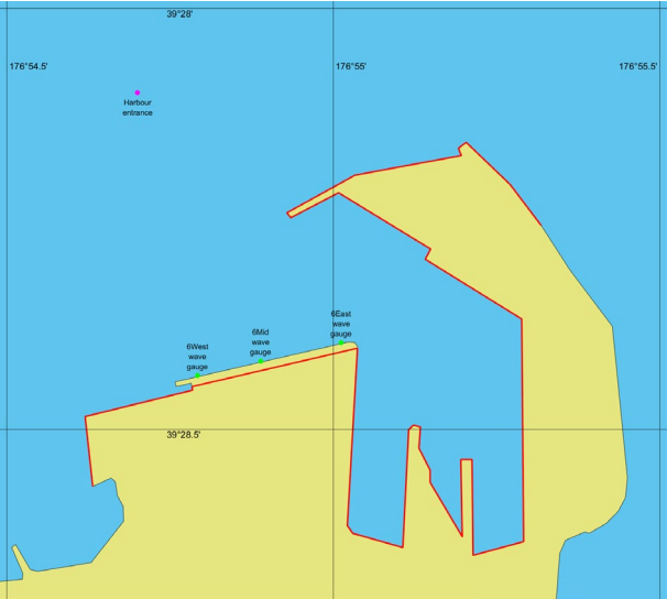
Figure 8 WAMIT harbour mesh (shown in red) for coupled ship-and-harbour method. Wave gauges at No. 6 Wharf shown in green. "Harbour entrance" modelling point shown in pink.
