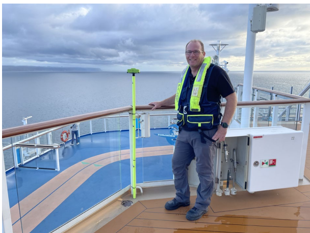
Figure 10 Capt. Robbie Jensen with starboard stern GNSS receiver on validation trials for Ovation of the Seas , 14 th Feb 2025. Similar receivers on the port side and bow allow survey-accuracy 6-DoF ship motions to be measured at 1 Hz.
