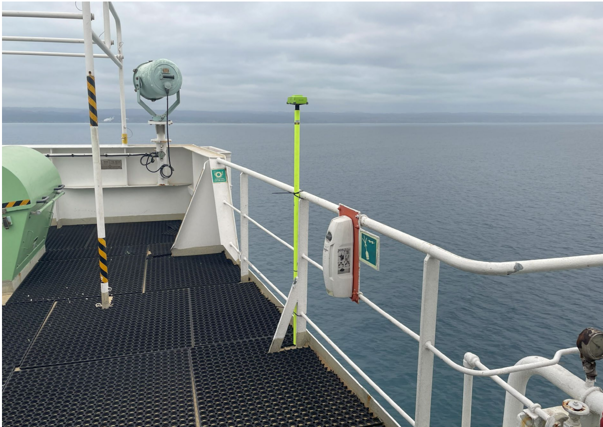
Figure 22: Starboard bridge wing GNSS receiver on Capitaine Baret
