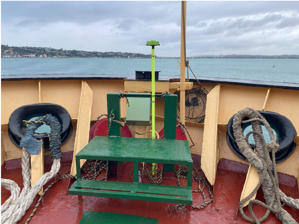
Figure 26: Bow GNSS receiver on Kota Lumba
