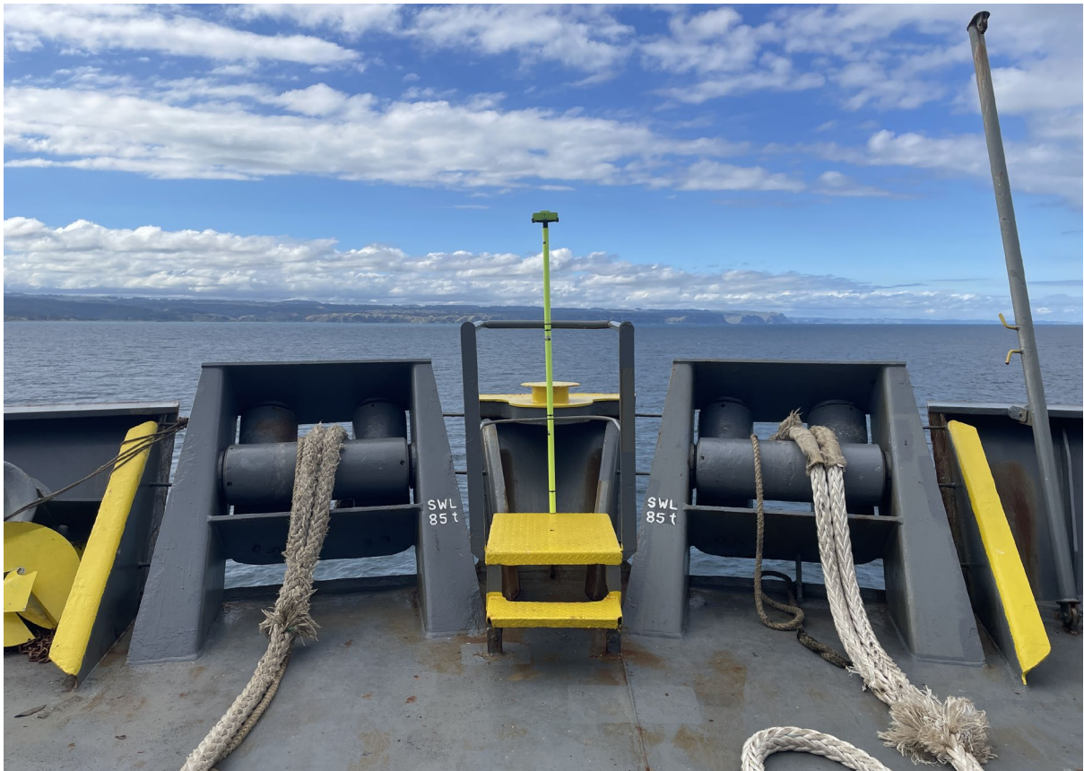
Figure 29: Bow GNSS receiver on NYK Futago
