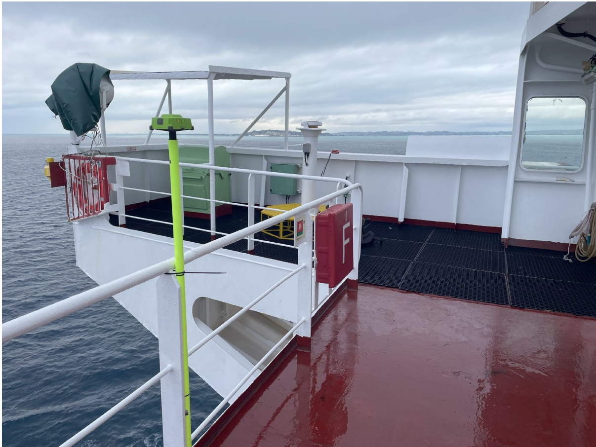
Figure 24: Port bridge wing GNSS receiver on Kota Lumba
