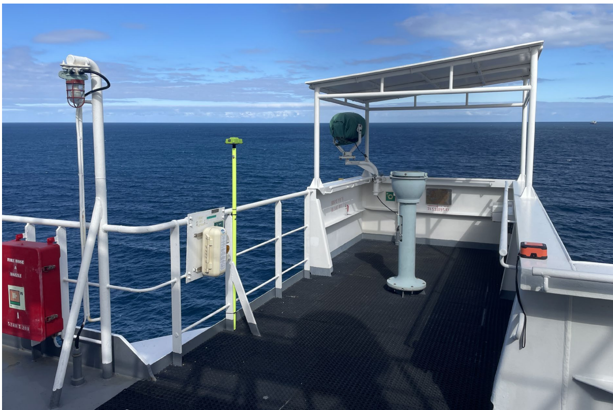
Figure 27: Port bridge wing GNSS receiver on NYK Futago
