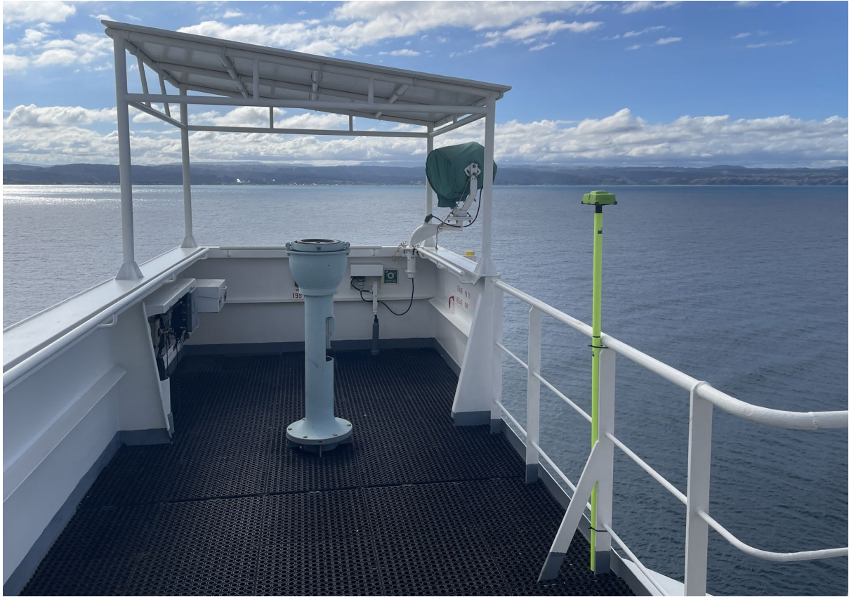
Figure 28: Starboard bridge wing GNSS receiver on NYK Futago
