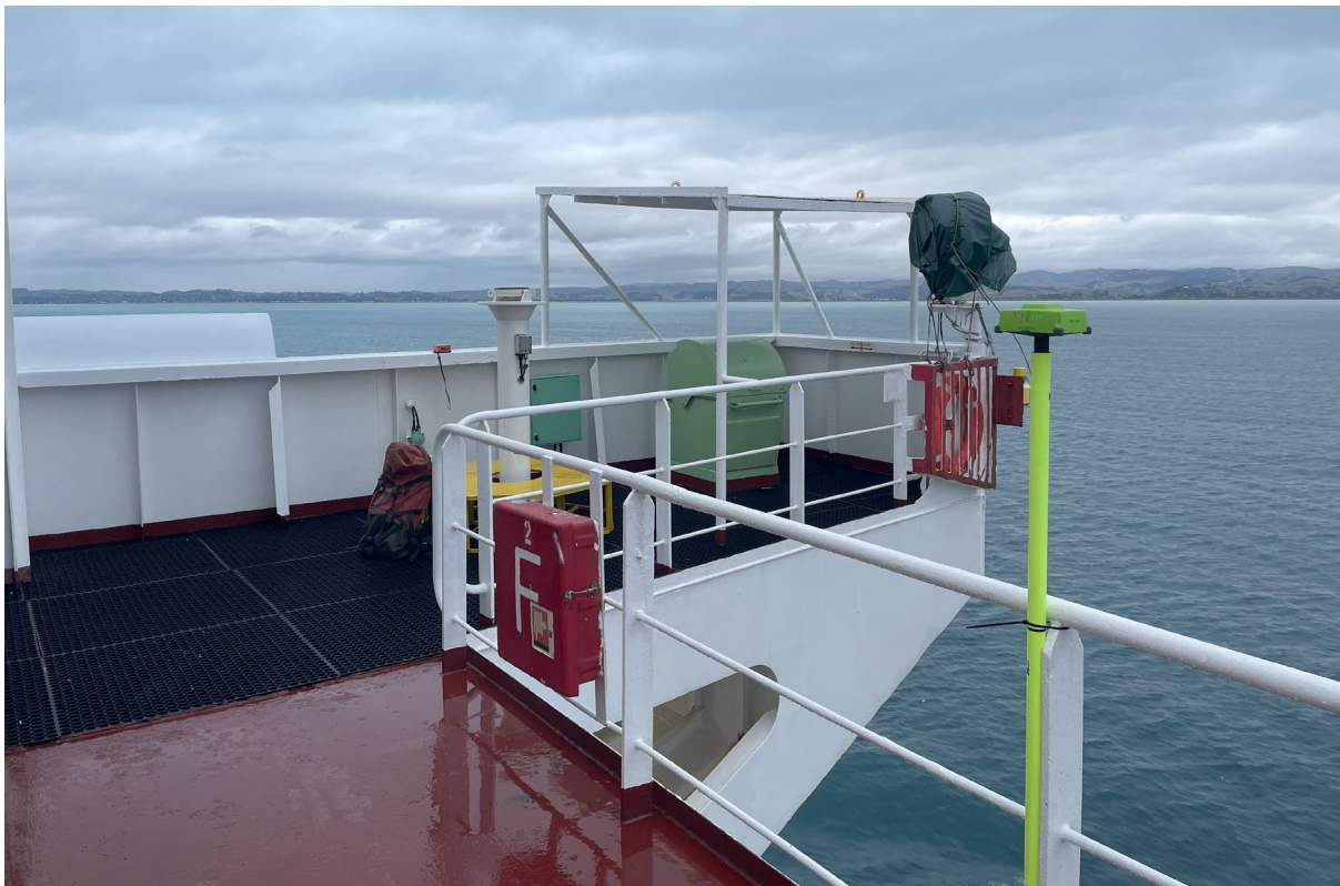
Figure 25: Starboard bridge wing GNSS receiver on Kota Lumba
