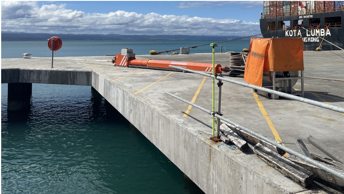
Figure 20: GNSS base station on west end of 6 Wharf, used for all GNSS measurements
