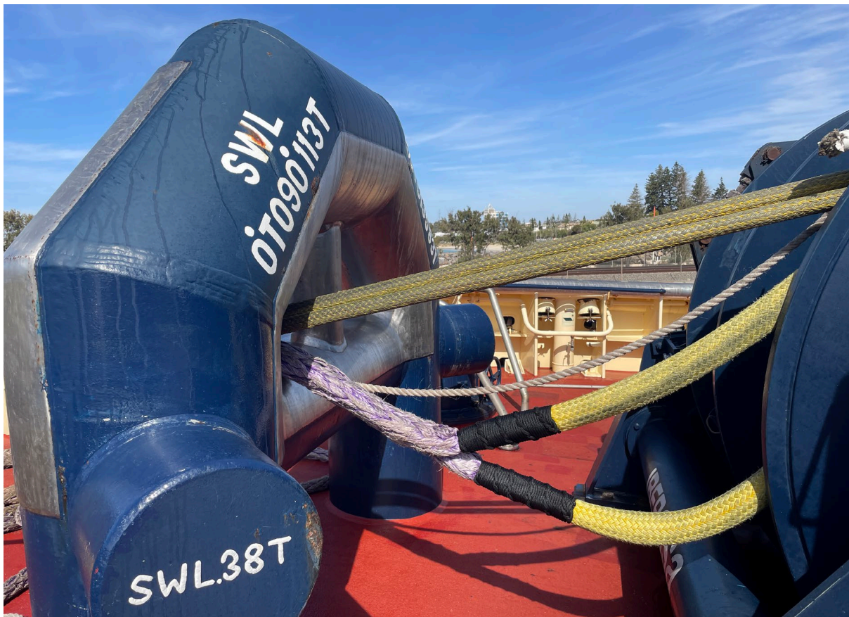
Figure 7: 24m towing pennant (purple plasma rope)
