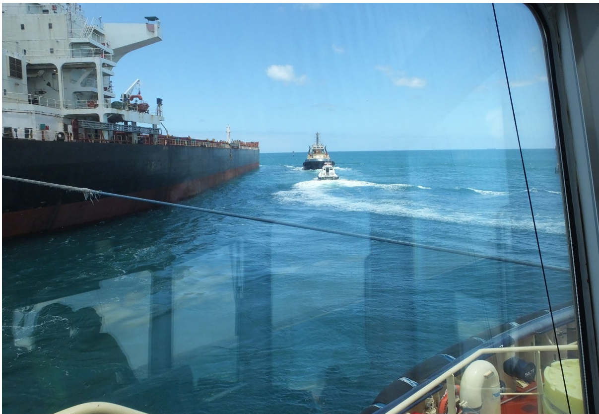
Figure 15: IMG_5347, taken 11:19, Bn11, indirect tow, speed 6 knots, line tension 20 tonnes, heel 6° to port, drift angle 45° to port
