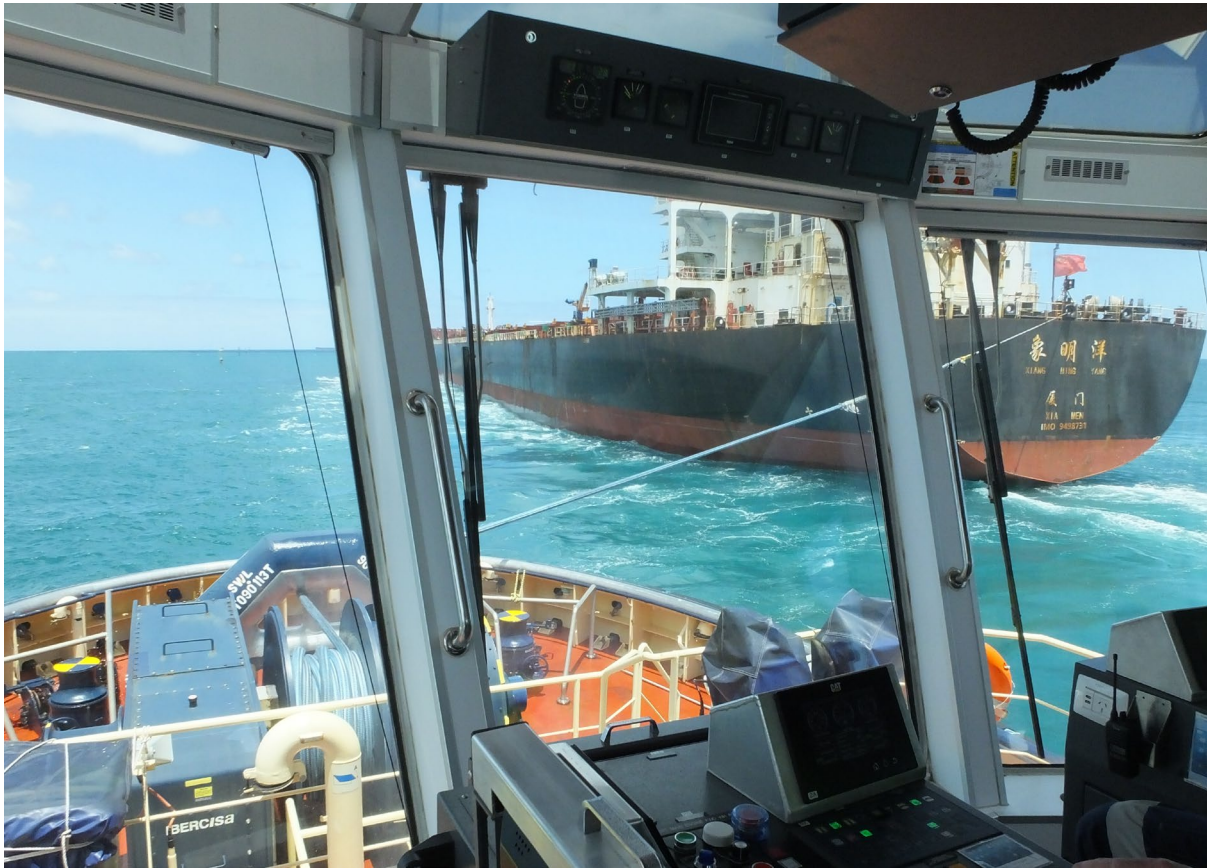
Figure 16: IMG_5350, taken 11:22, Bn9, speed 7 knots, line tension briefly 30 tonnes to arrest ship rate of turn, heel briefly 8° to starboard
