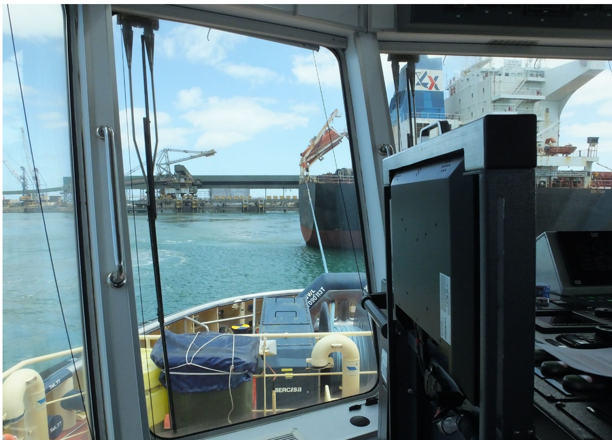
Figure 12: IMG_5321, taken 10:56, direct tow, speed 2 knots, line tension 40 tonnes, pitch 0.5° bow-up
