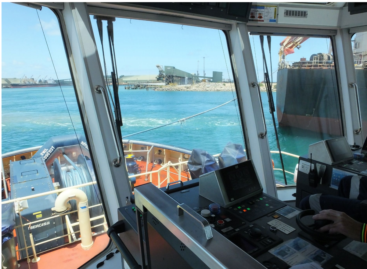
Figure 13: IMG_5331, taken 11:05, direct tow, speed 3 knots, line tension minimum
