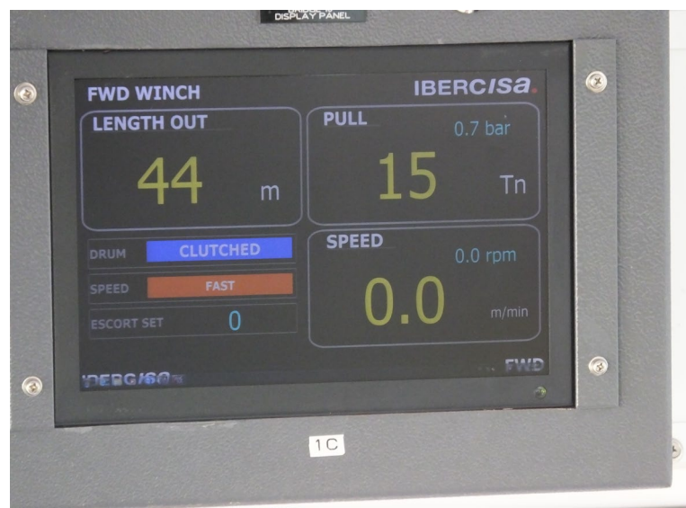
Figure 10: Svitzer North bridge display, showing line tension and length
