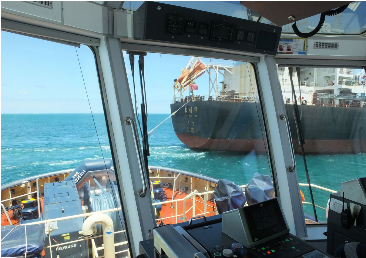
Figure 14: IMG_5339, taken 11:12, Bn 15-17, direct tow, speed 5 knots, line tension 30 tonnes, heel 2° to starboard, drift angle 90° to starboard
