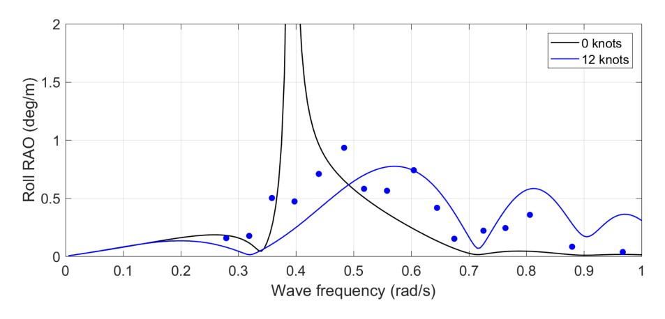
• Speed effect very important for inviscid and viscous damping, and encounter frequencies in following seas
