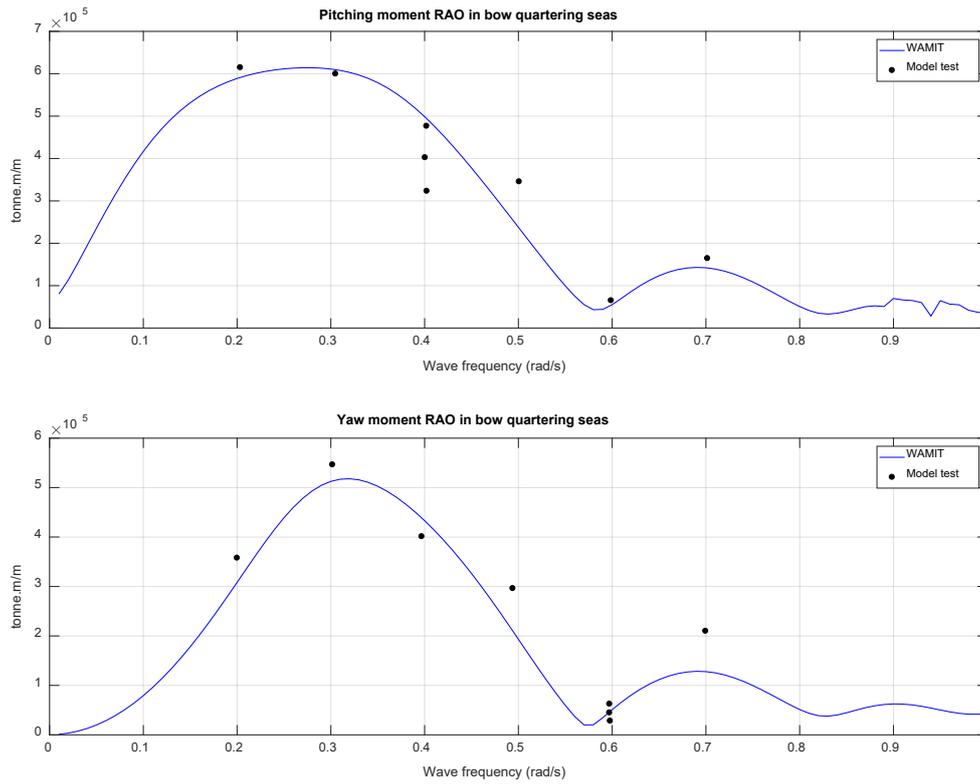
Figure 12: Wave heading 225° (port bow quartering seas): pitch and yaw wave-induced moment comparisons between WAMIT and model tests (van Oortmerssen 1976, Fig. 3.11).
