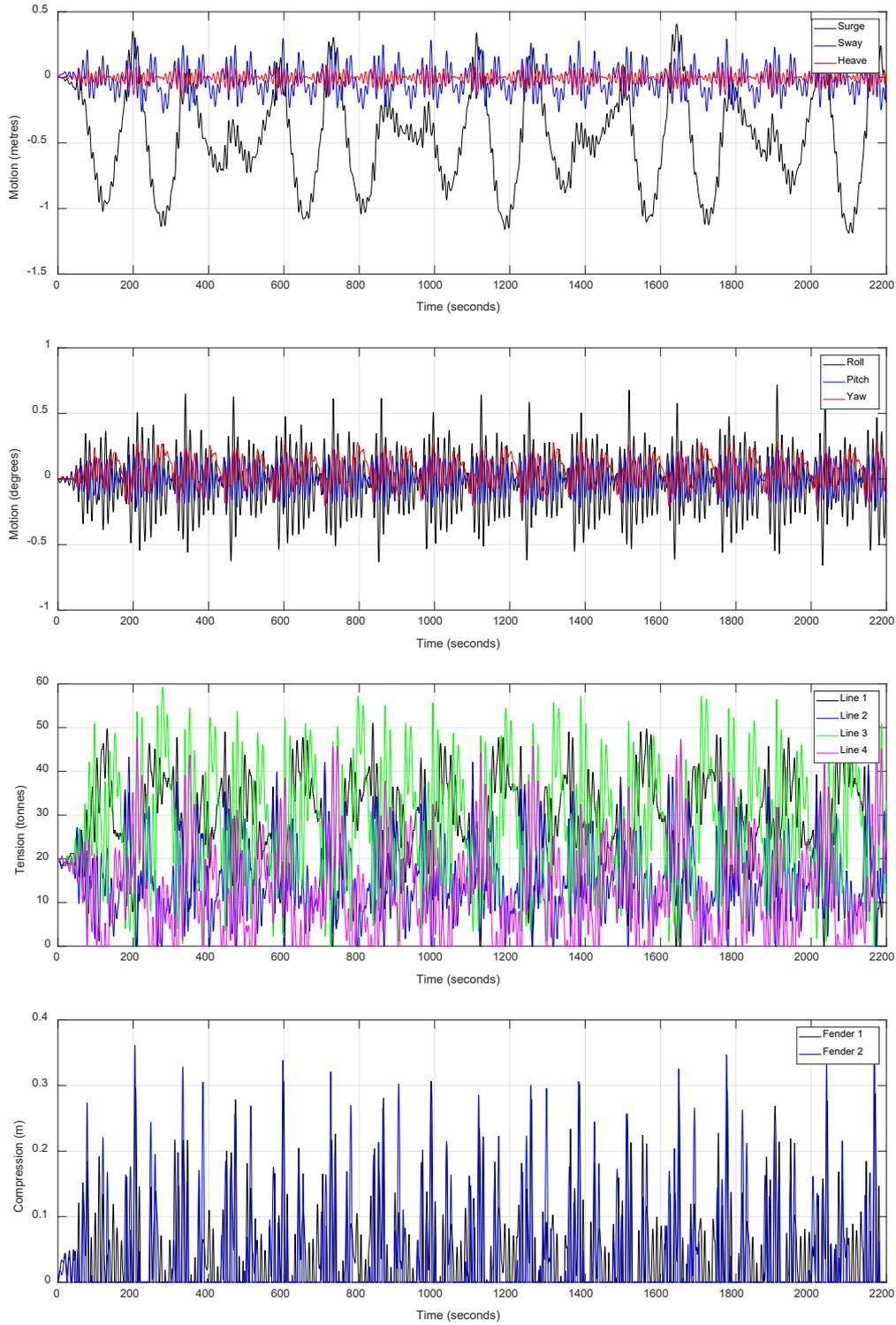
Figure 16: Motion and load timeseries for wave heading 135° (starboard bow quartering seas), irregular wave spectrum with  $H_s=2.6$  m
