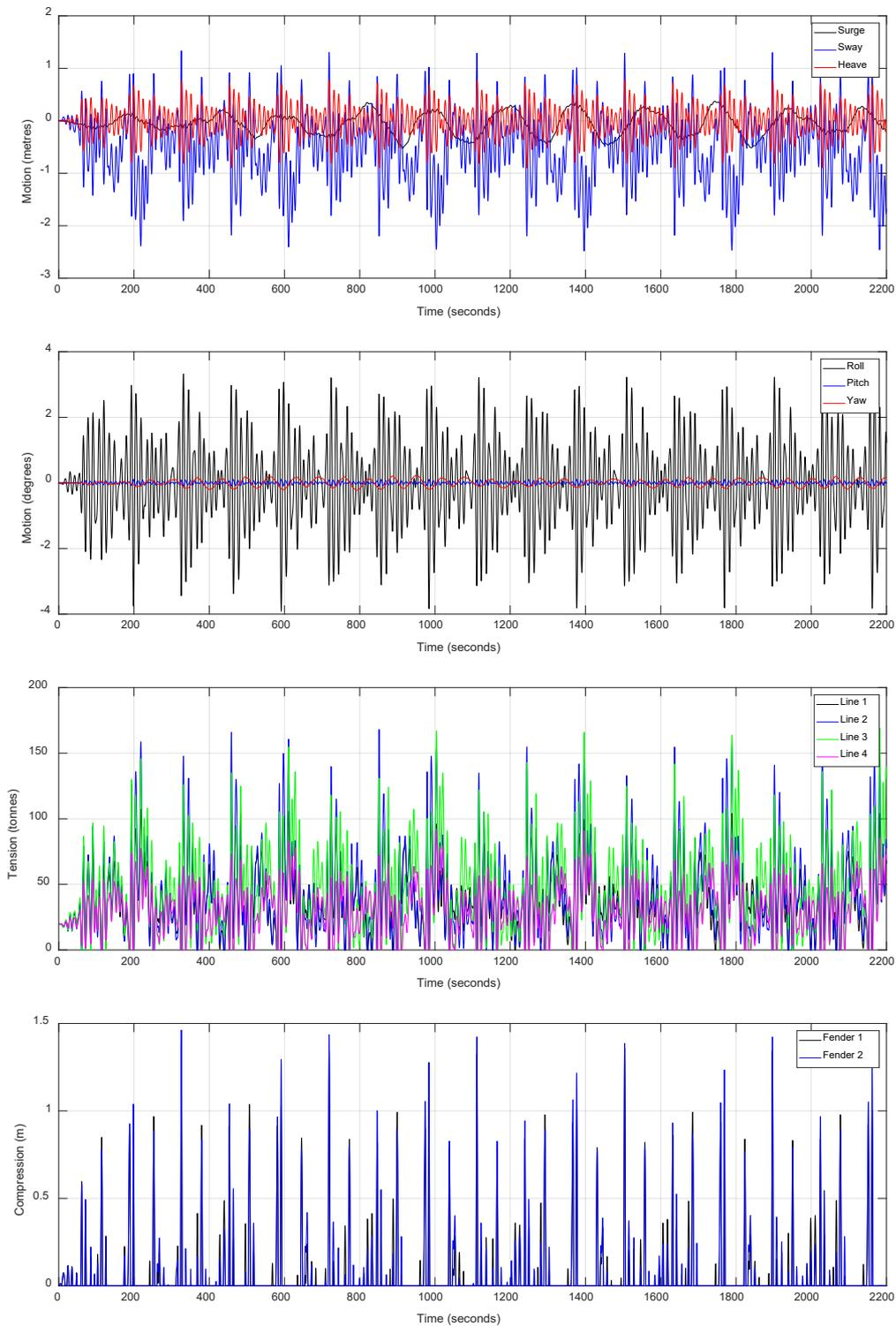
Figure 15: Motion and load timeseries for wave heading 90° (starboard beam seas), irregular wave spectrum with  $H_S=2.6$  m
