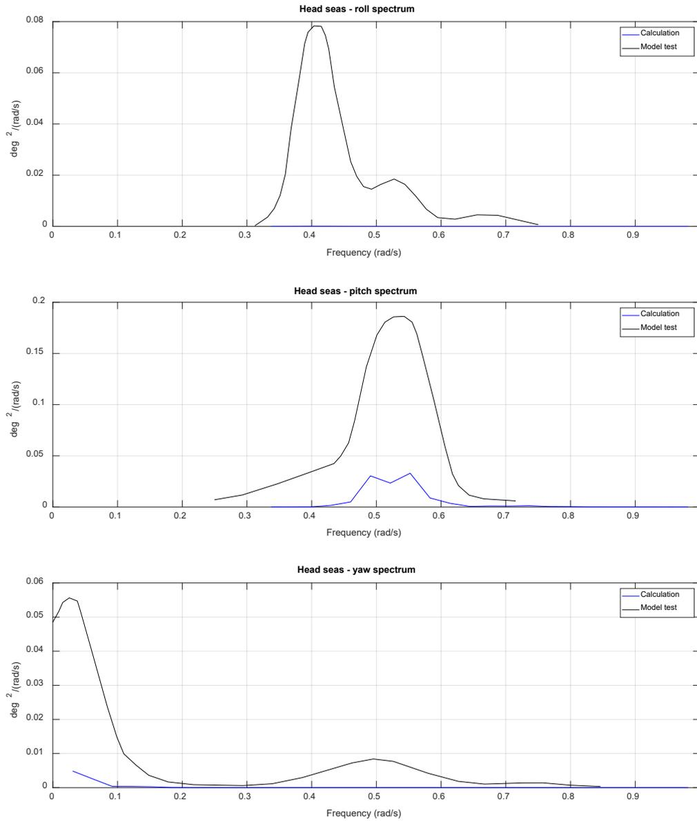
Figure 23: Wave heading 180° (head seas): roll, pitch and yaw spectra comparisons between MoorMotions and van Oortmerssen (1976, Fig. 5.12)
