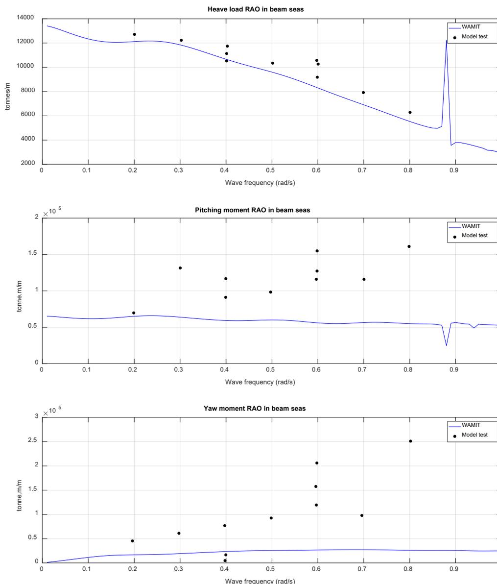
**Figure 14: Wave heading 270° (port beam seas): heave, pitch and yaw wave load comparisons between WAMIT and model tests (van Oortmerssen 1976, Fig. 3.12).**
