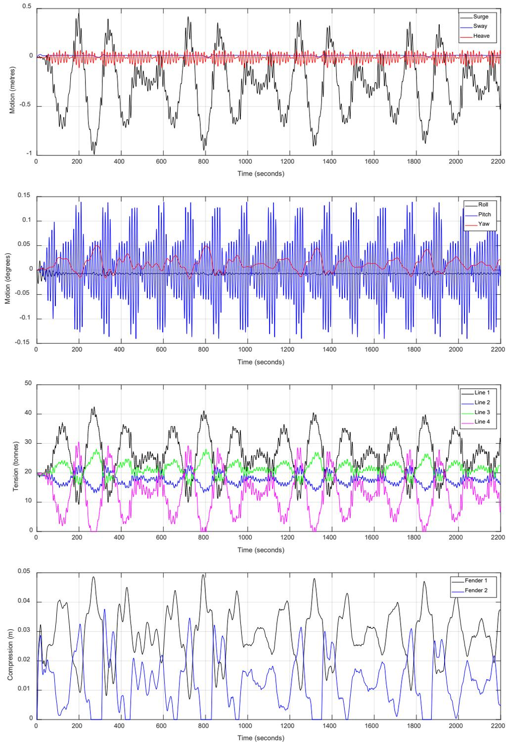
Figure 17: Motion and load timeseries for wave heading 180° (head seas), irregular wave spectrum with  $H_s=2.6$  m
