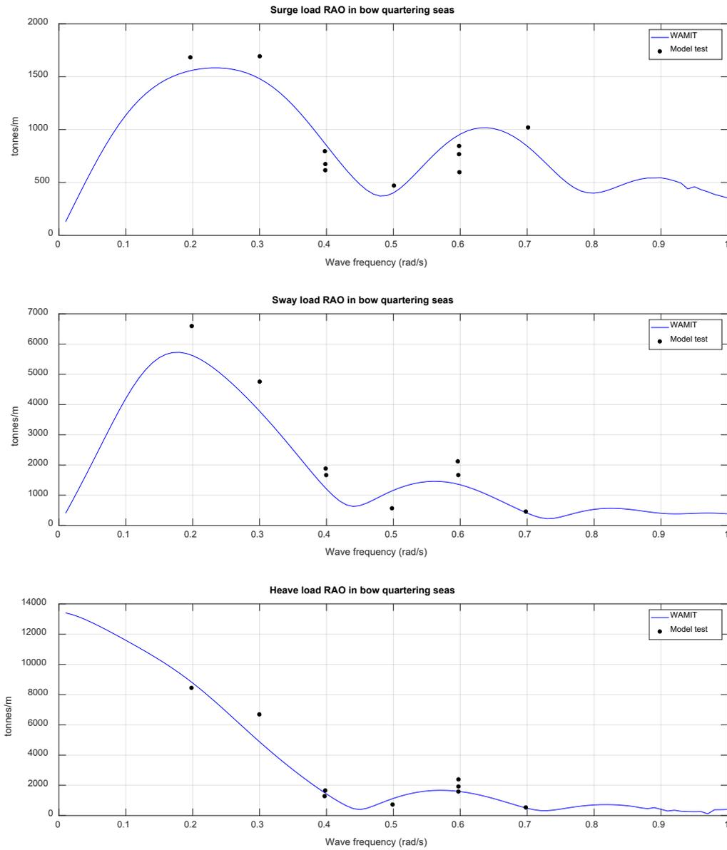
Figure 11: Wave heading 225° (port bow quartering seas): surge, sway and heave wave load comparisons between WAMIT and model tests (van Oortmerssen 1976, Fig. 3.11).
