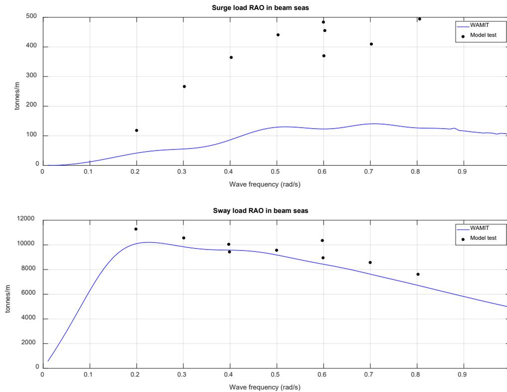
Figure 13: Wave heading 270° (port beam seas): surge and sway wave load comparisons between WAMIT and model tests (van Oortmerssen 1976, Fig. 3.12).
