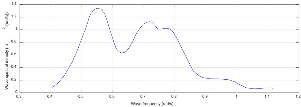
**Figure 2: Wave spectrum used for moored ship model tests (van Oortmerssen 1976, Fig. 5.9). Significant wave height is 2.6 m.**
