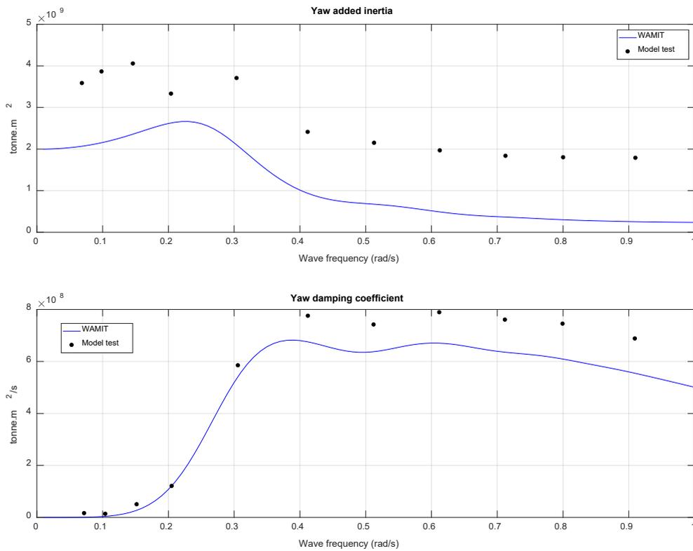
Figure 9: Yaw hydrodynamic coefficient comparisons between WAMIT and model tests (van Oortmerssen 1976, Fig. 3.18).
