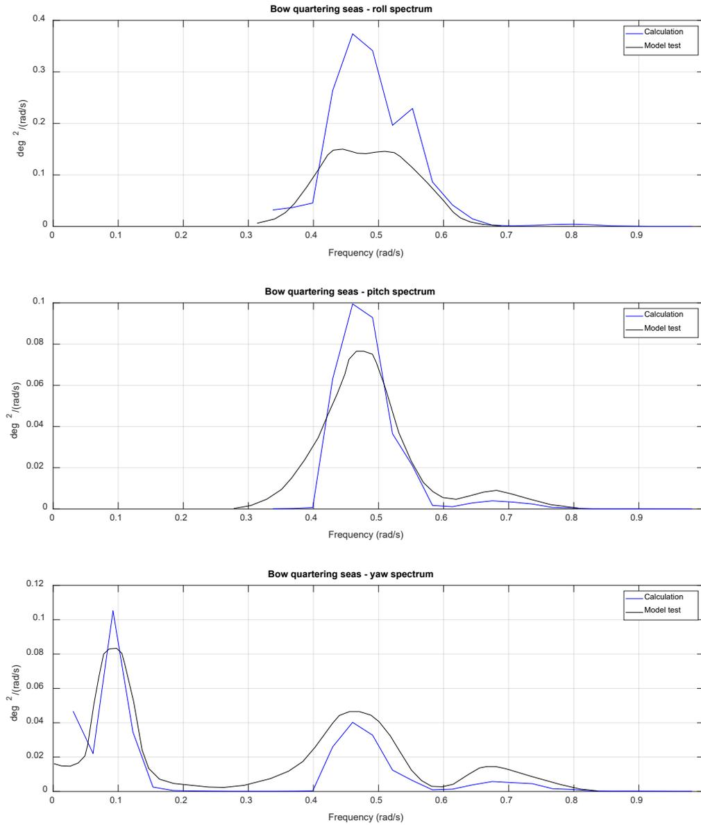
Figure 21: Wave heading 135° (starboard bow quartering seas): roll, pitch and yaw spectra comparisons between MoorMotions and van Oortmerssen (1976, Fig. 5.11)
