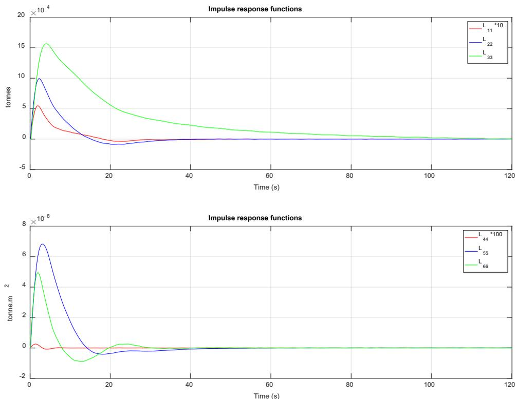
Figure 4: Diagonal impulse response functions  $L_{ii}(t)$  for 200,000 DWT tanker in shallow water
