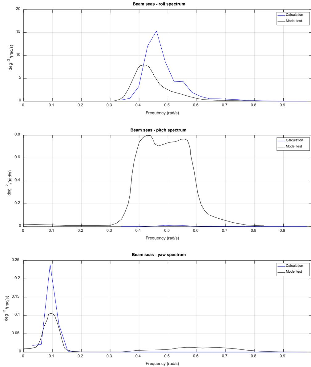
**Figure 19: Wave heading 90° (starboard beam seas): roll, pitch and yaw spectra comparisons between MoorMotions and van Oortmerssen (1976, Fig. 5.10)**
