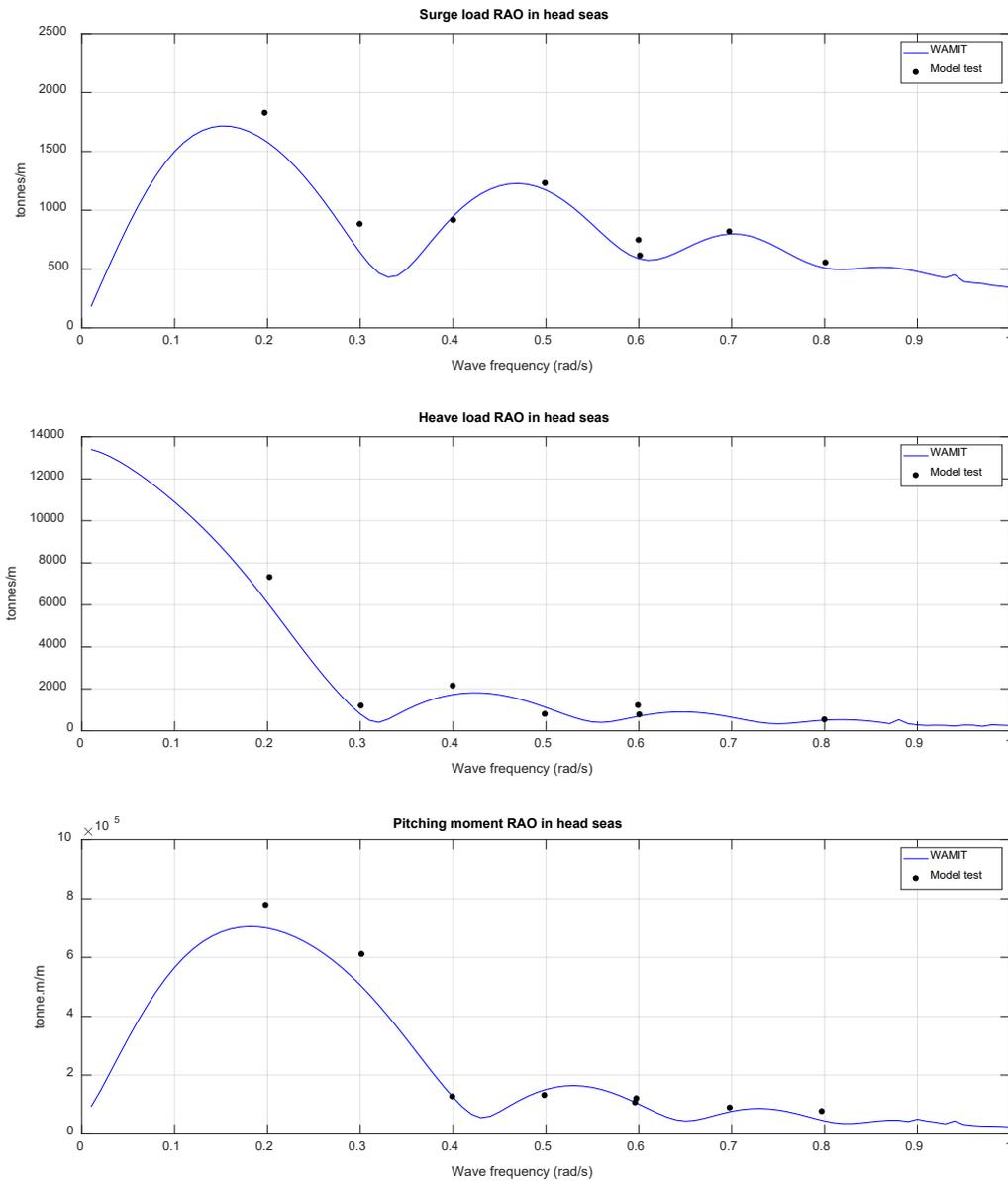
Figure 10: Wave heading 180° (head seas): wave load comparisons between WAMIT and model tests (van Oortmerssen 1976, Fig. 3.10).
