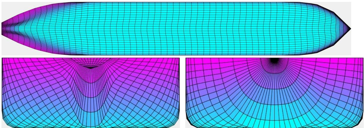
**Figure 3: 200,000 DWT tanker surface mesh, up to design waterline. (Top) Plan view; (Bottom left) Stern view; (Bottom right) Bow view.**
