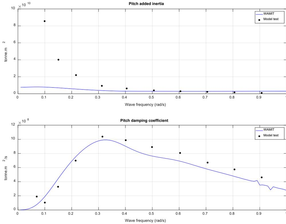
Figure 8: Pitch hydrodynamic coefficient comparisons between WAMIT and model tests (van Oortmerssen 1976, Fig. 3.17).
