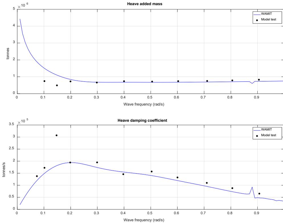
Figure 7: Heave hydrodynamic coefficient comparisons between WAMIT and model tests (van Oortmerssen 1976, Fig. 3.15).
