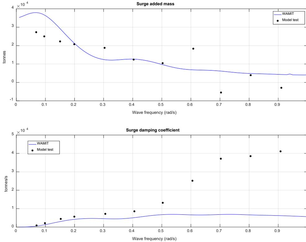
Figure 5: Surge hydrodynamic coefficient comparisons between WAMIT and model tests (van Oortmerssen 1976, Fig. 3.13).
