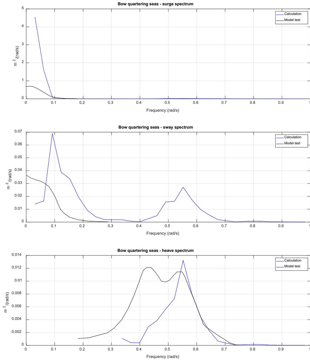
Figure 20: Wave heading 135° (starboard bow quartering seas): surge, sway and heave spectra comparisons between MoorMotions and van Oortmerssen (1976, Fig. 5.11)
