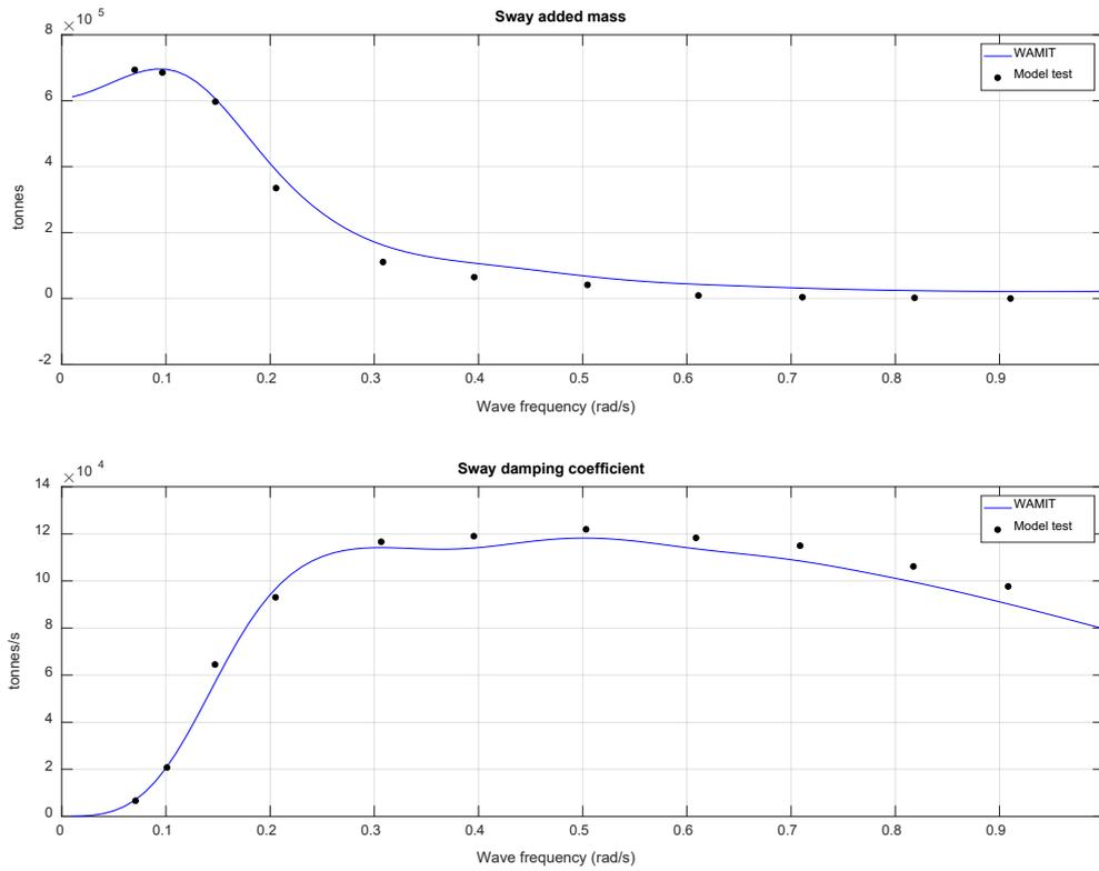
Figure 6: Sway hydrodynamic coefficient comparisons between WAMIT and model tests (van Oortmerssen 1976, Fig. 3.14).
