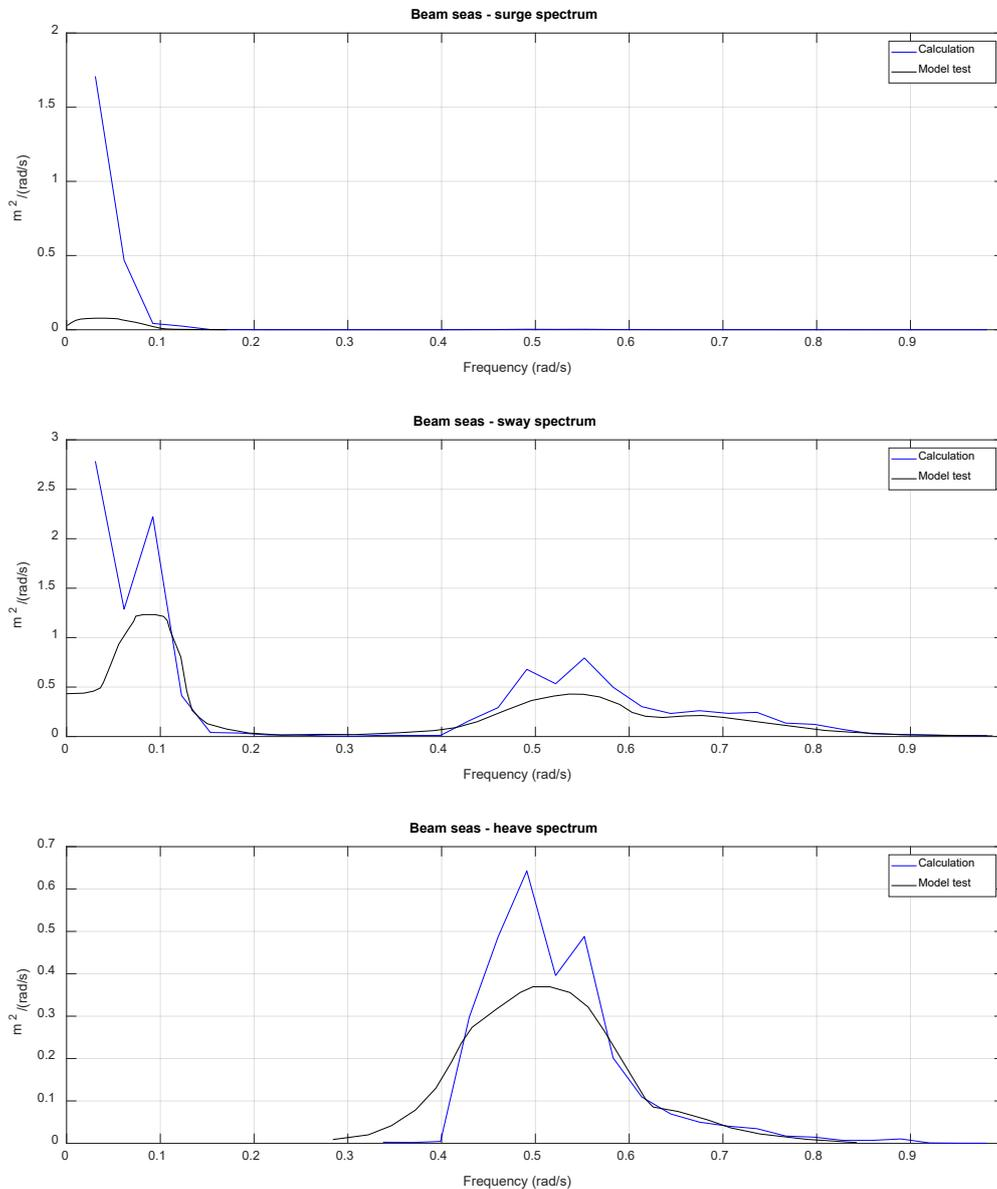
Figure 18: Wave heading 90° (starboard beam seas): surge, sway and heave spectra comparisons between MoorMotions and van Oortmerssen (1976, Fig. 5.10)
