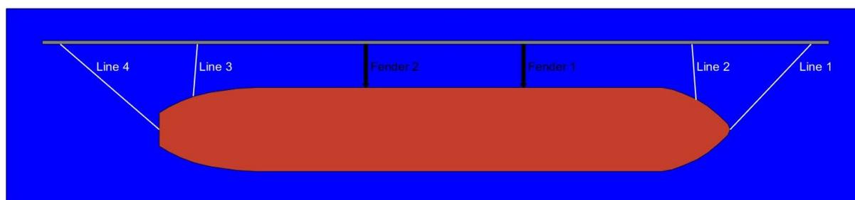
**Figure 1: Mooring arrangement used for model testing of 200,000 DWT tanker, from van Oortmerssen (1976, Figs. 5.2, 5.4, 5.5)**
