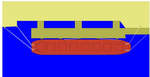
Figure 6 Mooring arrangement for Sea Diamond at Berth 5, 1<sup>st</sup> – 2<sup>nd</sup> Oct 2015. Shore bollard positions taken from Geraldton Harbour chart. Ship plan and mooring gear positions taken from ship General Arrangement.
