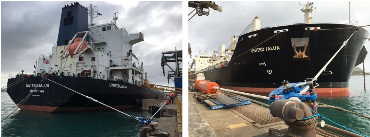
Figure 14: United Jalua ShoreTension trials at berth 3. Photo MWPA
