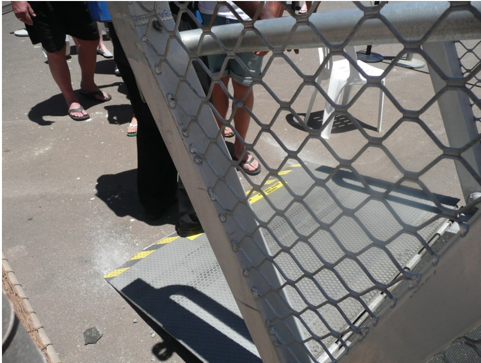
Figure 17: Passengers boarding Pacific Sun, moored at Geraldton berth 6. Note scraping of ramp on concrete due to ship movement, and passenger footwear. Photo MWPA.
