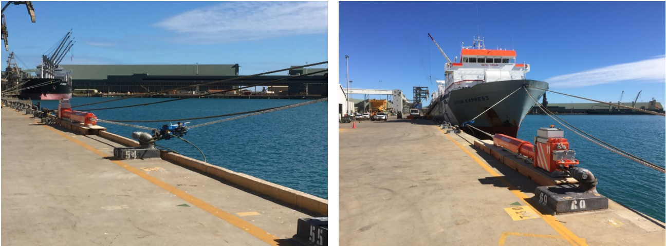
Figure 15: Bison Express ShoreTension trials at berth 2. Photo MWPA
