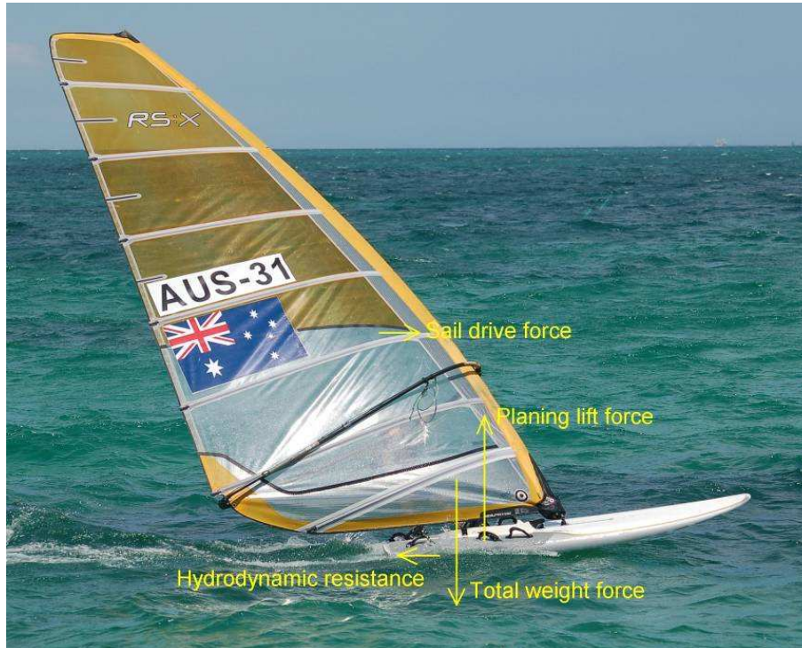
Figure 8: Planing upwind - pitch moment balance
