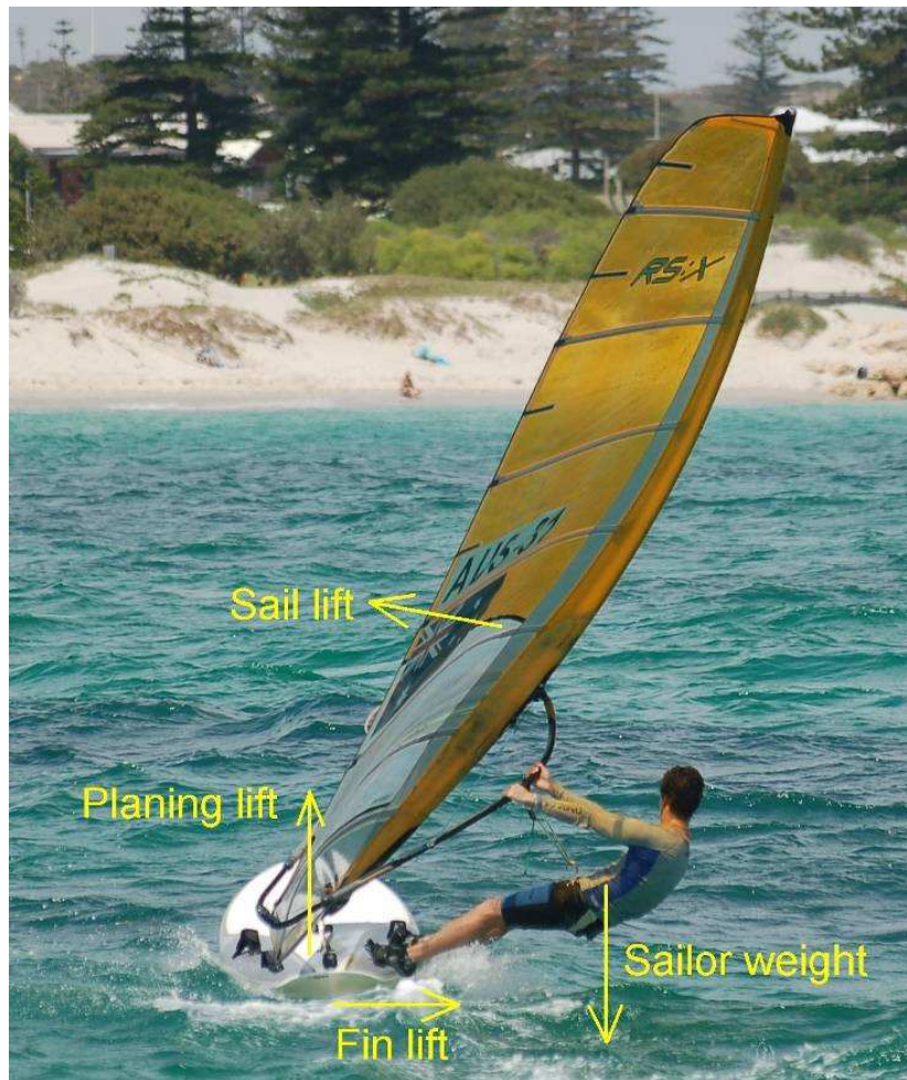
Figure 4: Planing upwind: main transverse and vertical forces
