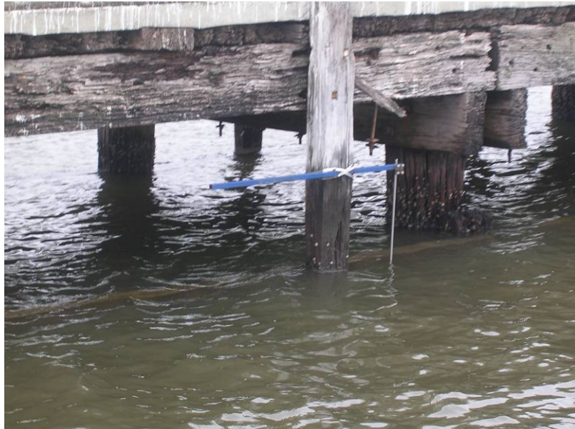
Figure 3: Submerged waverecorder attached to old Ellam St jetty
