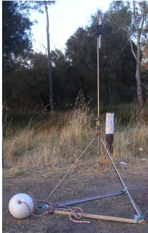
Figure 1: Submerged seabed-mounted frame used at Ashfield Parade, with waverecorder attached to top
