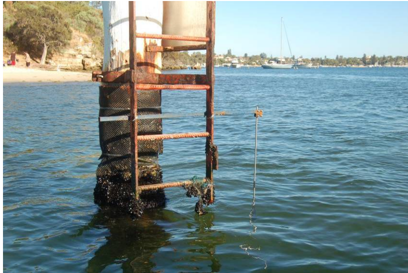
Figure 4: Submerged waverecorder attached to frame mounted on Chidley Point pilon
