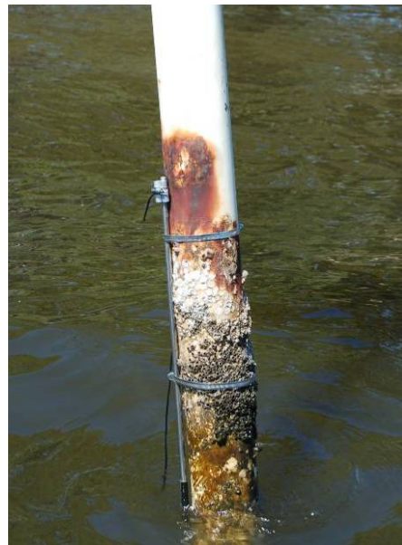
Figure 5: Submerged waverecorder attached directly to Goodwood Parade pilon
