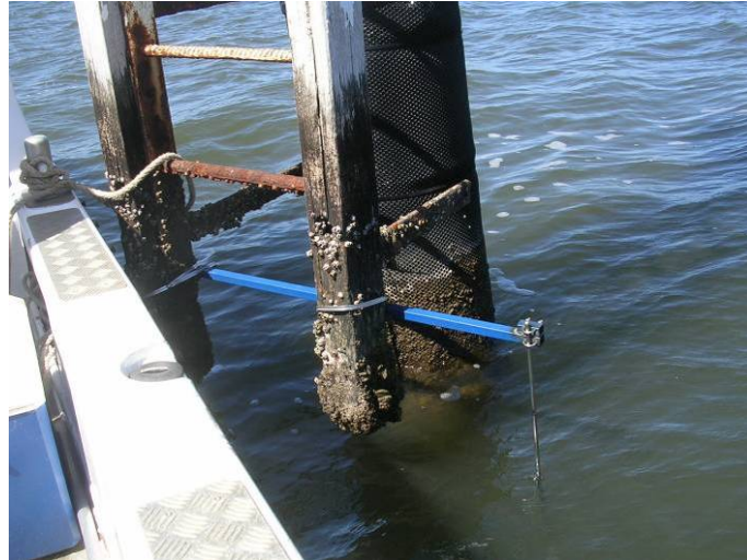
Figure 2: Submerged waverecorder attached to frame mounted on Quarry Point pilon
