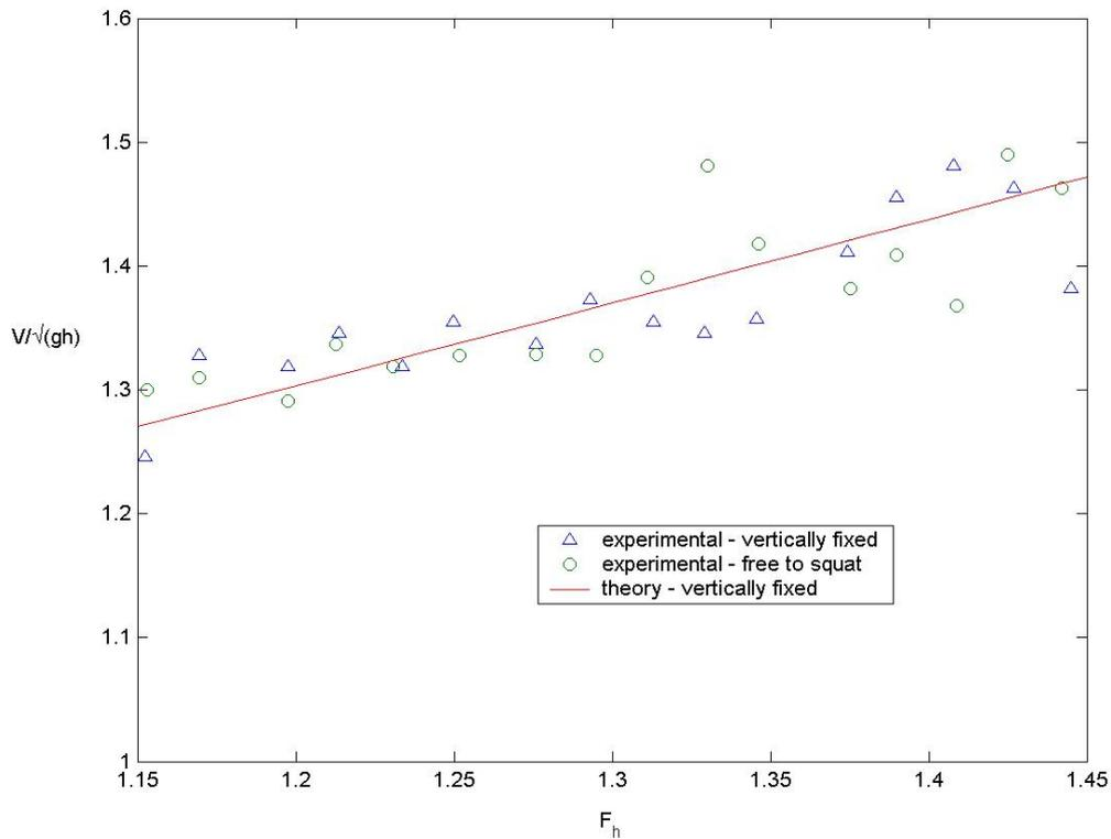
Fig. 4: Scaled bore speed  $V/\sqrt{gh}$  as a function of  $F_h$ ; theory and experiment
